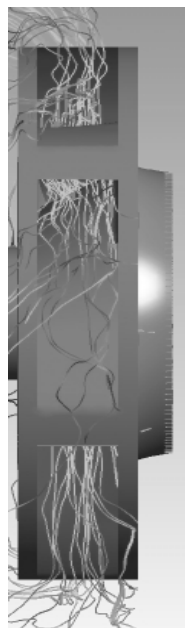
Fig. 7. Visualization of the streamlines in the radial impeller of centrifugal pumps.
