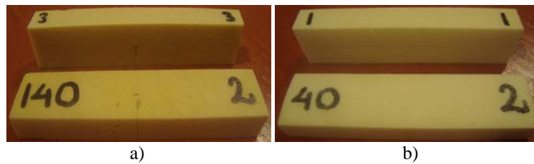
Fig. 4. Shape of the specimens used for 3PB tests: a) ELR; b) DF.
