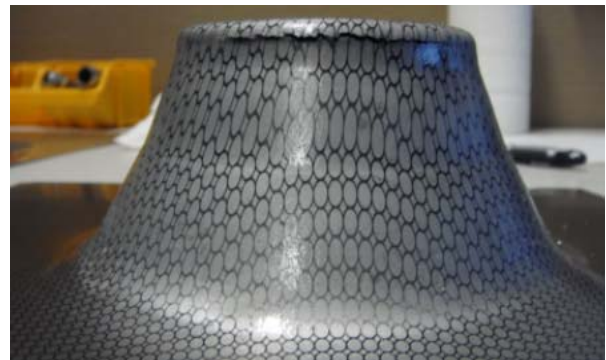
Fig. 6 Part formed according to the second geometry, t_0 = 1\text{mm} .
