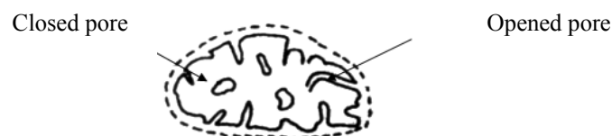
Fig. 6. Conceptual figure of a solid particle with opened and closed pores [20].
